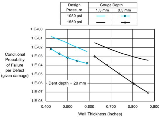
Figure 7 Conditional Annual Probability of Failure of Dent/Gouge
