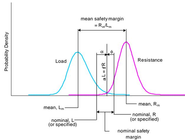
Figure 2 Load and Resistance Probability Distributions
