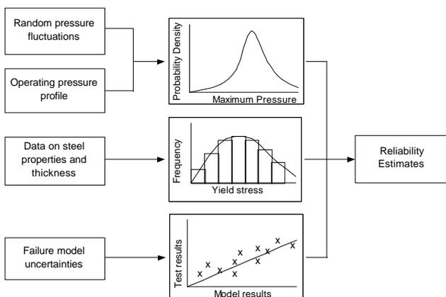
Figure 1 Reliability-based Design Concept for Internal Pressure
