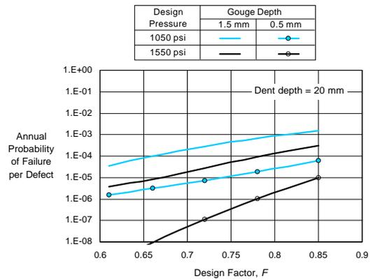
Figure 8 Annual Probability of Failure of Dent/Gouge
