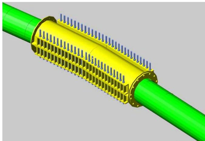
**Figure 10 - Repair Sleeve**
