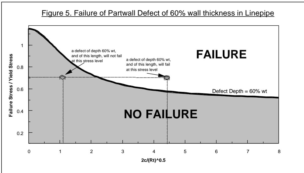
You can see that defects of constant depth, will either fail, or not fail, depending on their length, at the various stress levels.
