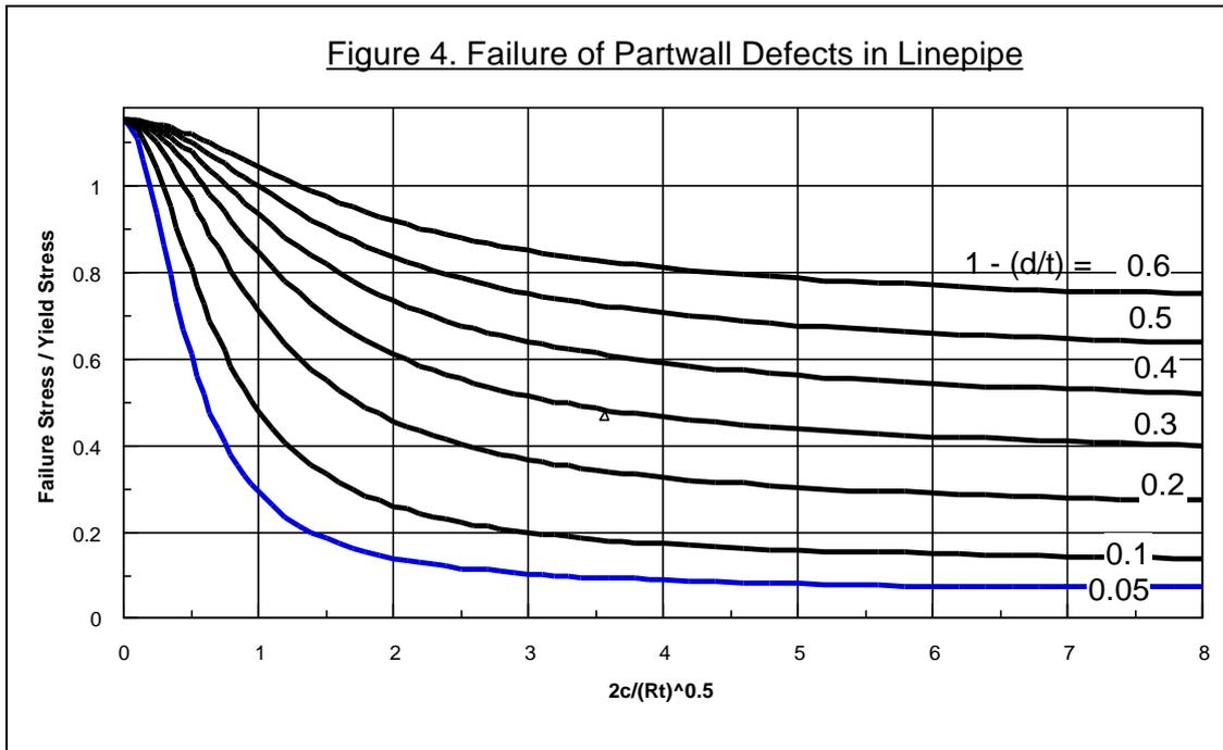
It is important to understand how the above curves work. The following example illustrates what these curves tell us. In this case, we are plotting the failure curve for a defect of depth 60% wall thickness (this gives us a remaining ligament  $(1 - d/t)$  of 0.4, see Figure 4)
