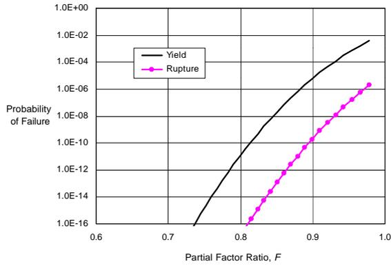
Figure 3 Annual Probability of Failure Due to Internal Pressure of New Pipe
