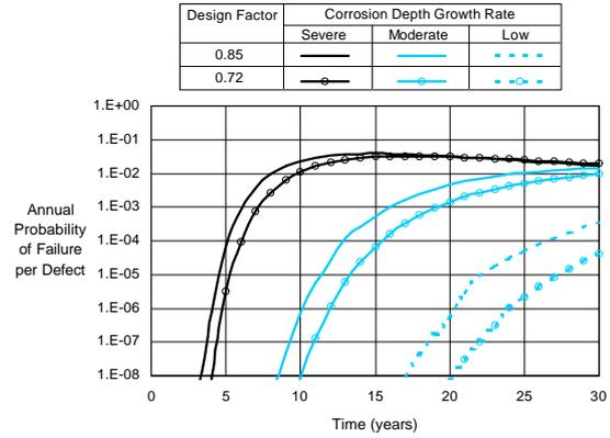
Figure 4 Annual Probability of Failure of Corroded Pipe (Combined Leaks and Ruptures)
