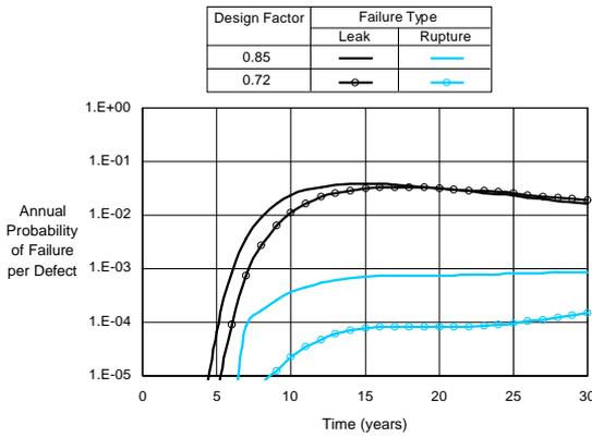
Figure 5 Annual Probability of Failure - Severe Corrosion Rate (0.25 mm/yr)
