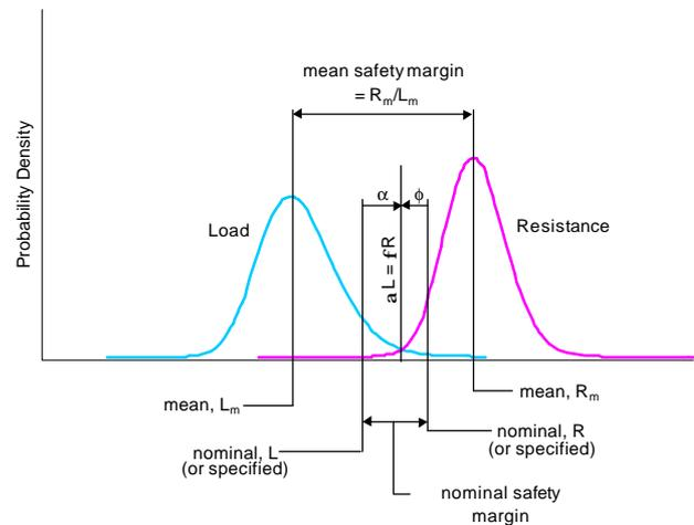
Figure 2 Load and Resistance Probability Distributions
