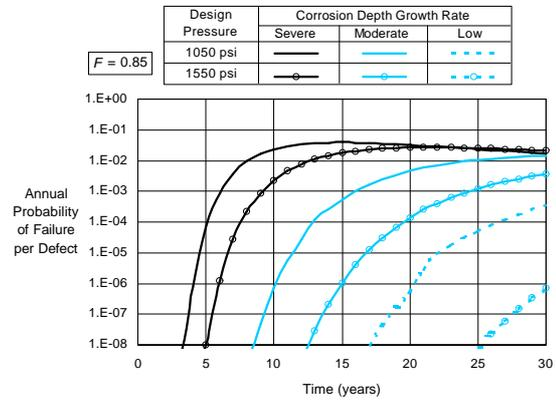
Figure 6 Annual Probability of Failure - Effect of Higher Pressure ( $F = 0.85$ )
