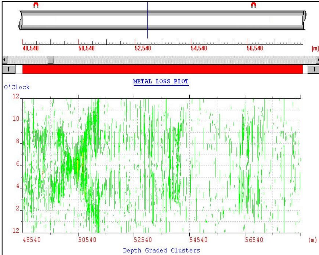
Figure E1 – General Corrosion Plot and Magnet Positions for Section of Pipeline
