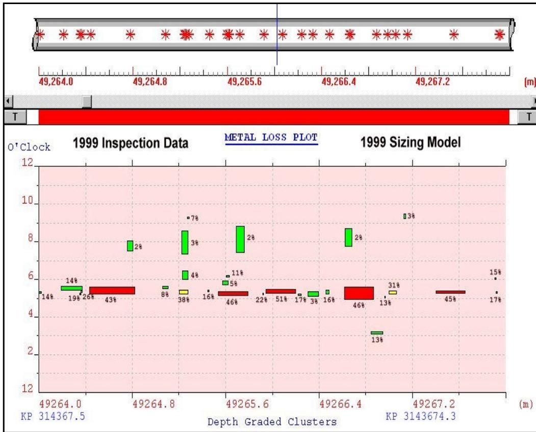
Figure C1 – 1999 Inspection Data, Assessed Using 1999 Sizing Model
