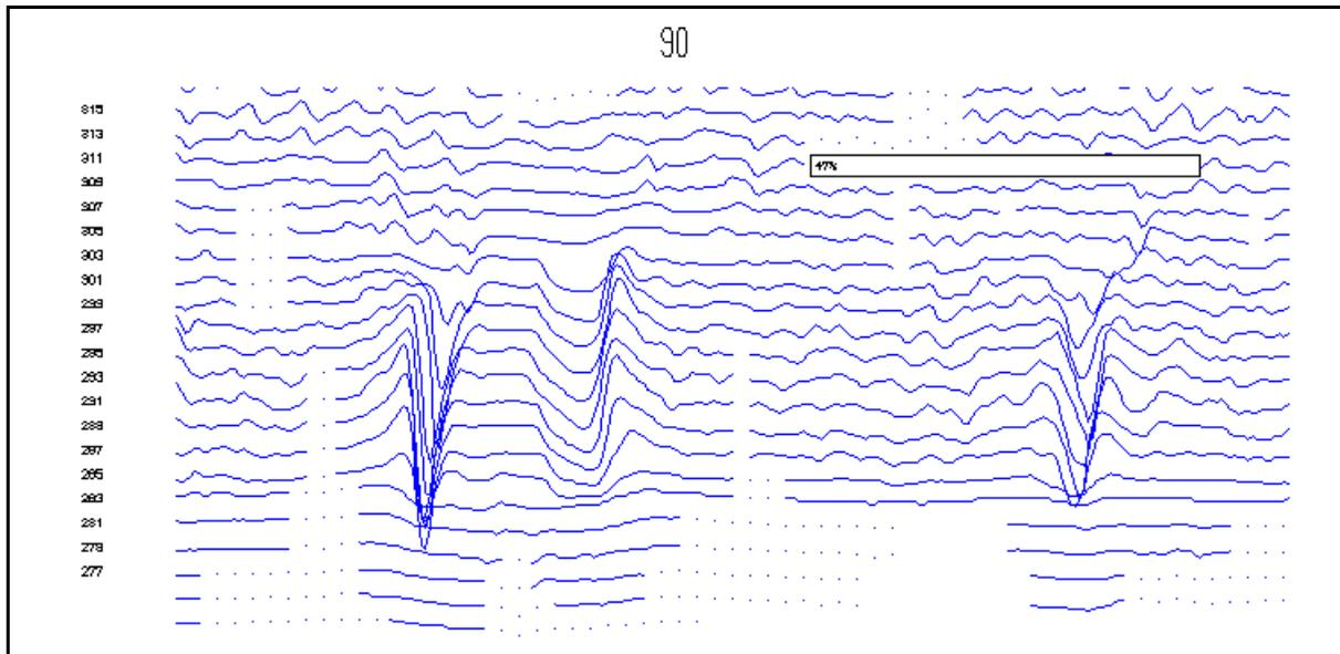
Figure B1 – Magnetic Flux Leakage Signal, Worst Defects, 1990
