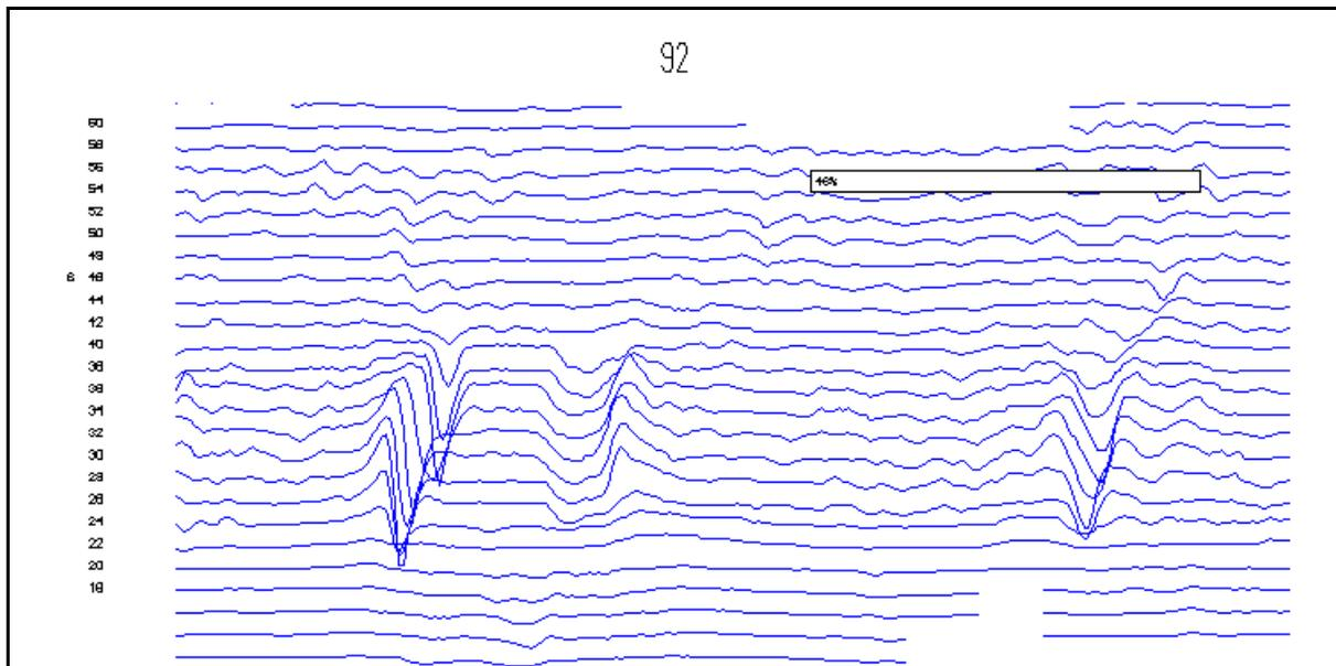
Figure B2 – Magnetic Flux Leakage Signal, Worst Defects, 1992
