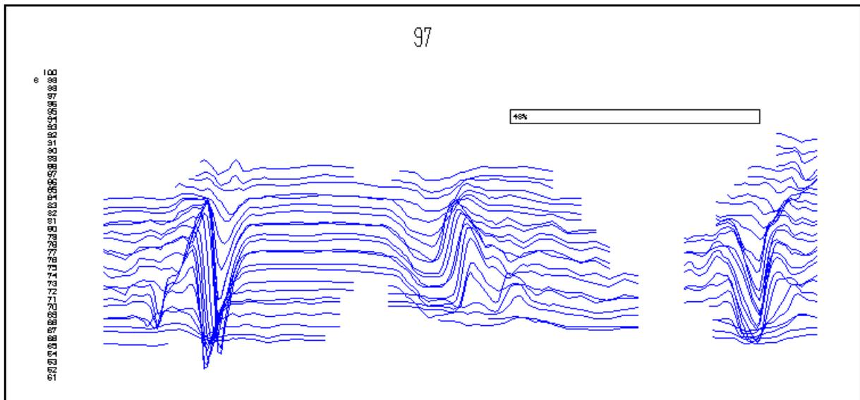
**Figure B4 – Magnetic Flux Leakage Signal, Worst Defects,1997**
