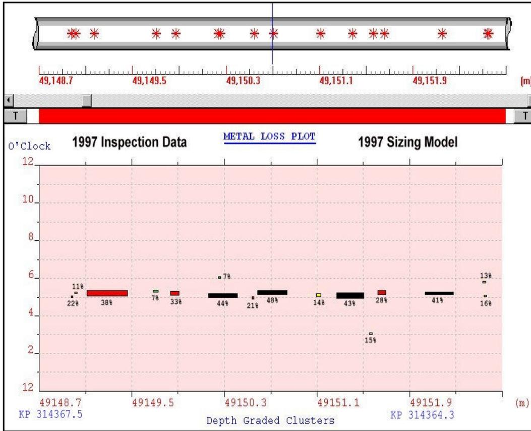
Figure C2 – 1997 Inspection Data, Assessed Using 1997 Sizing Model
