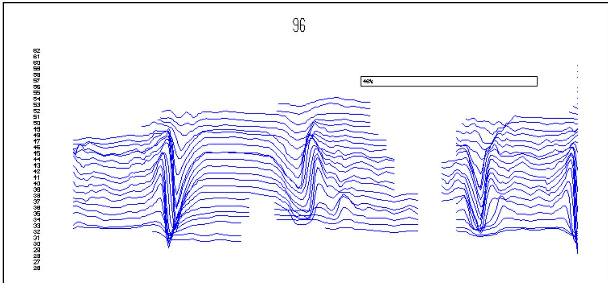
**Figure B3 – Magnetic Flux Leakage Signal, Worst Defects,1996**
