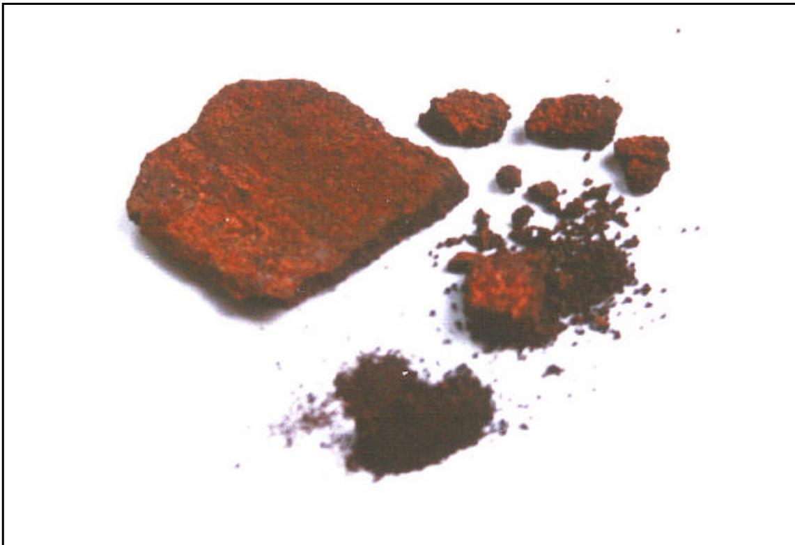
**Figure G3 – Sample of Debris Crust Removed from the Pipe**
