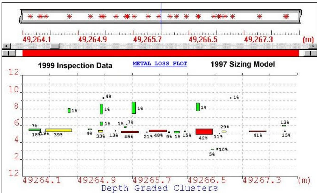
Figure C3 – 1999 Inspection Data, Re-assessed Using 1997 Sizing Model
