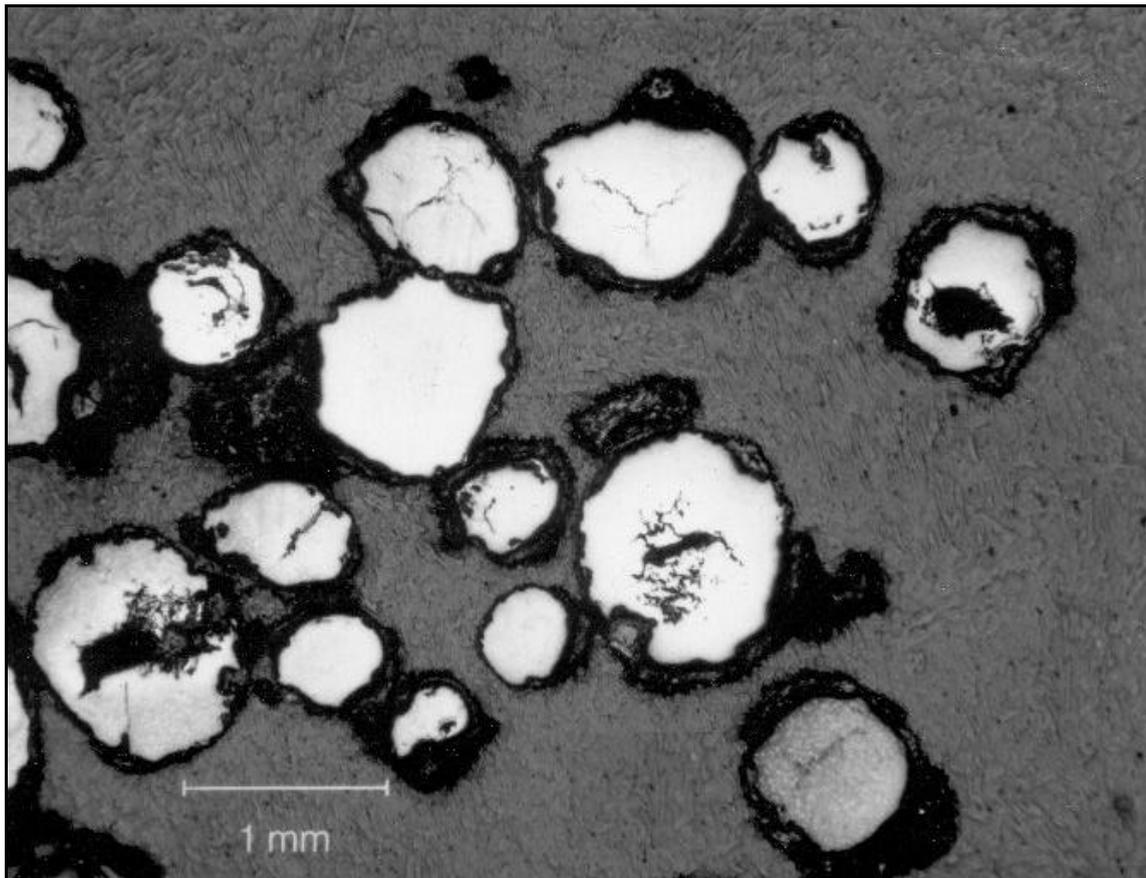
**Figure G4 – Microscopic Close-Up of Sectioned Debris Material**
