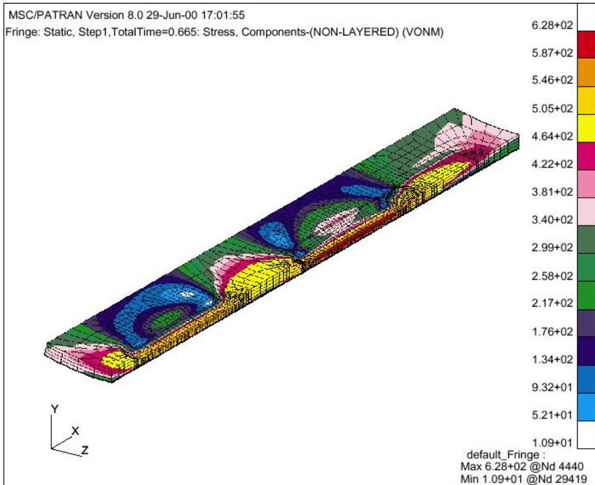
Figure D1 – Von Mises Stress Distribution for Worst Defect Combination
