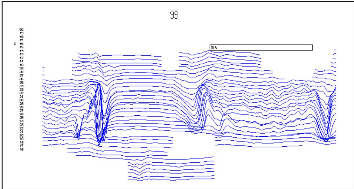
**Figure B5 – Magnetic Flux Leakage Signal, Worst Defects,1999**
