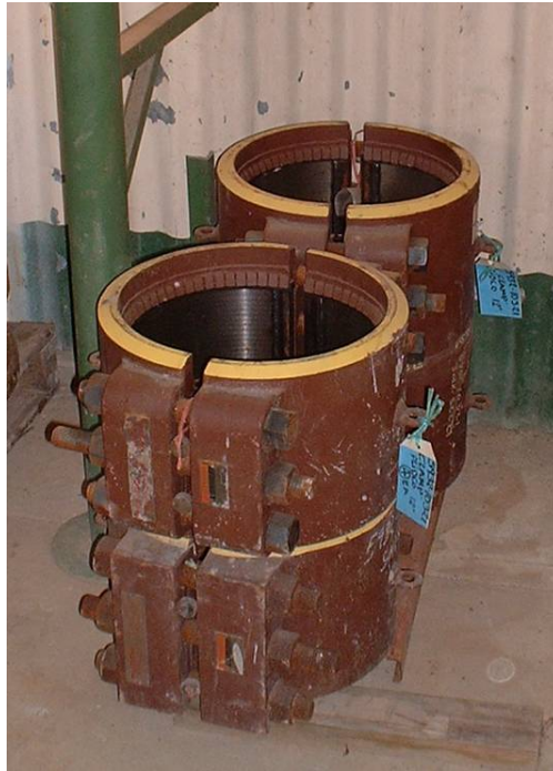
Figure 8 Bolted Clamp Repairs
