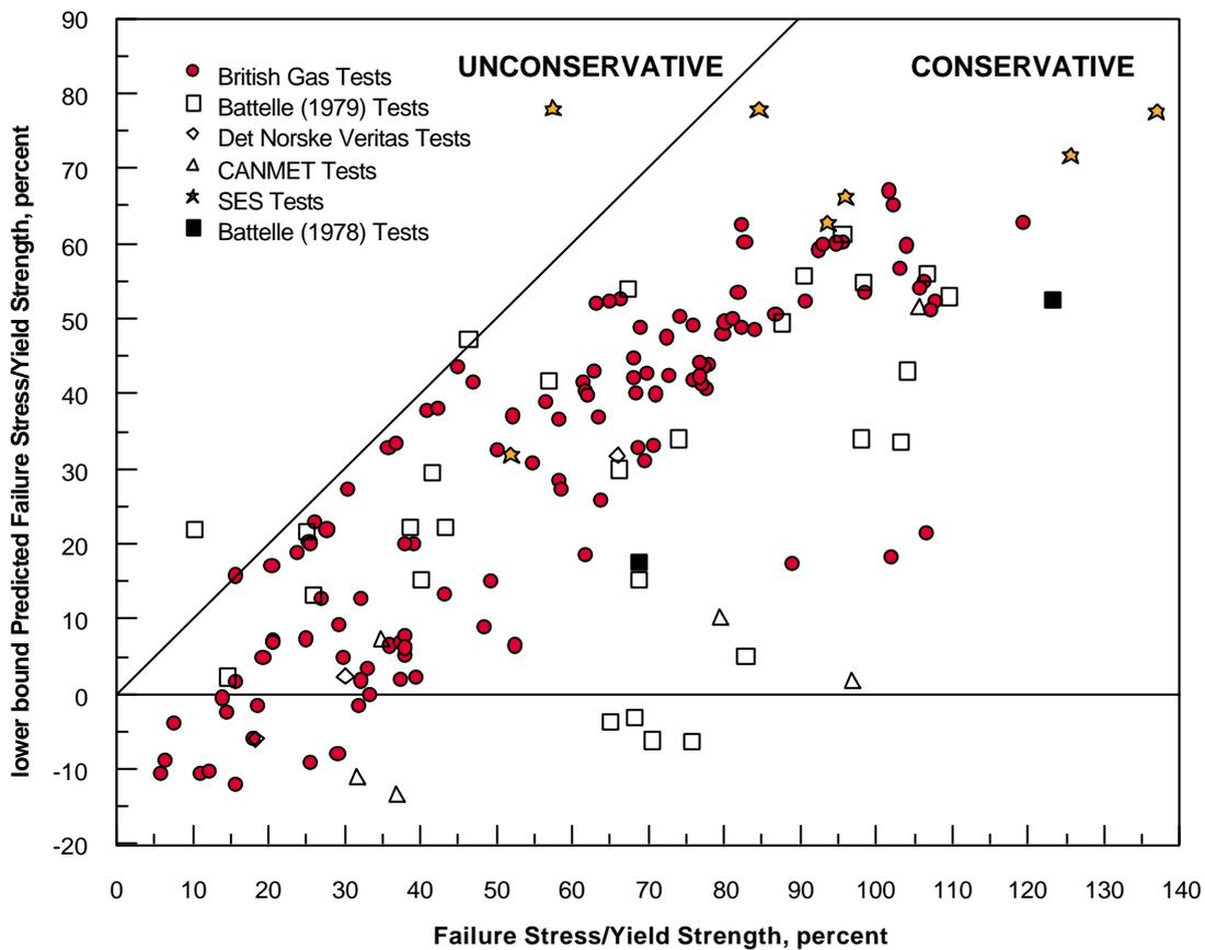
**Figure 9 – Failure stress of dent and gouge defects predicted using a lower bound to the dent-gouge fracture model**
