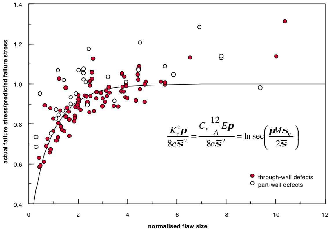
**Figure 1 – Summary of the early work at Battelle leading to the development of the NG-18 equations**
