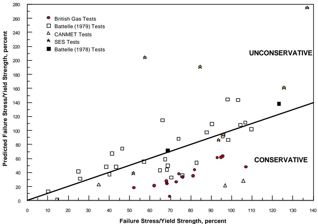
**Figure 7 – Failure stress of dent and gouge defects predicted using the empirical Q factor model**
