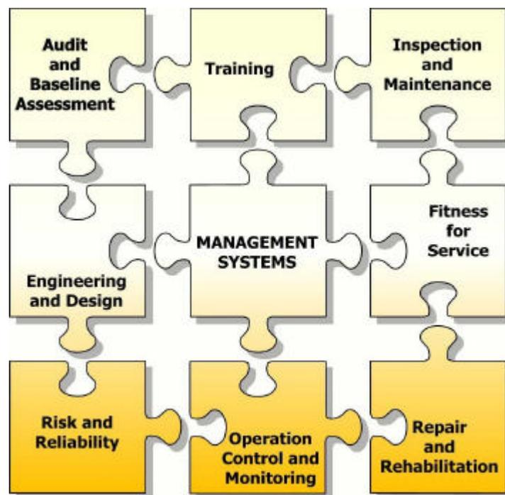
**Figure 10 – The Key Elements of Pipeline Integrity Management**
