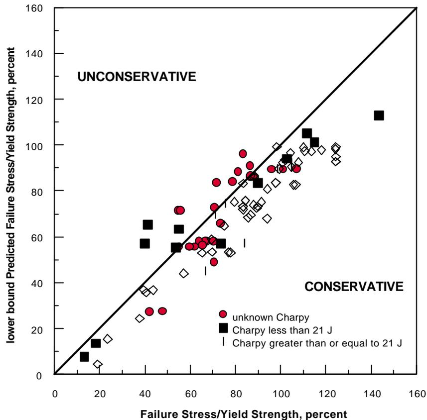
**Figure 6 – Failure stress of axially orientated part-wall defects predicted using a lower bound to the part-wall NG-18 equations**
