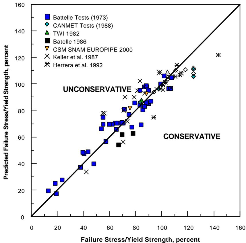
**Figure 4 – Failure stress of axially orientated part-wall defects predicted using the part-wall NG-18 equations**
