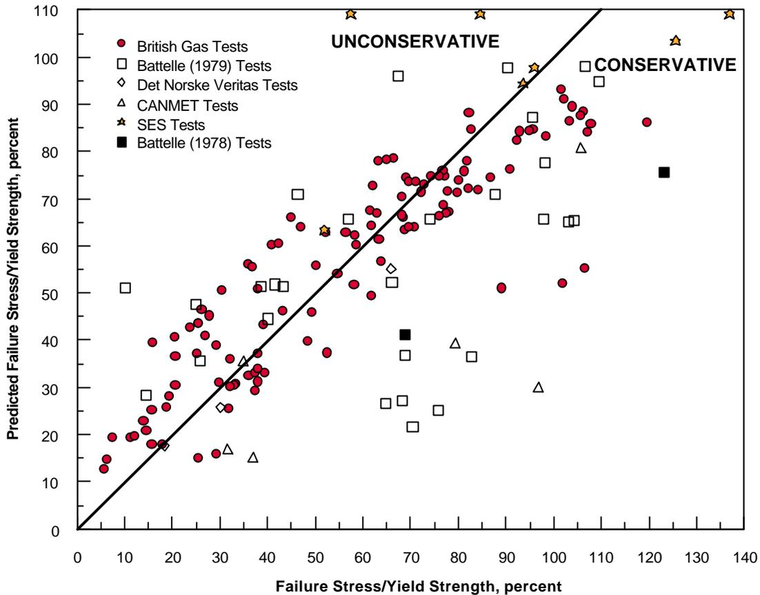
**Figure 8 – Failure stress of dent and gouge defects predicted using the semi-empirical dent-gouge fracture model**
