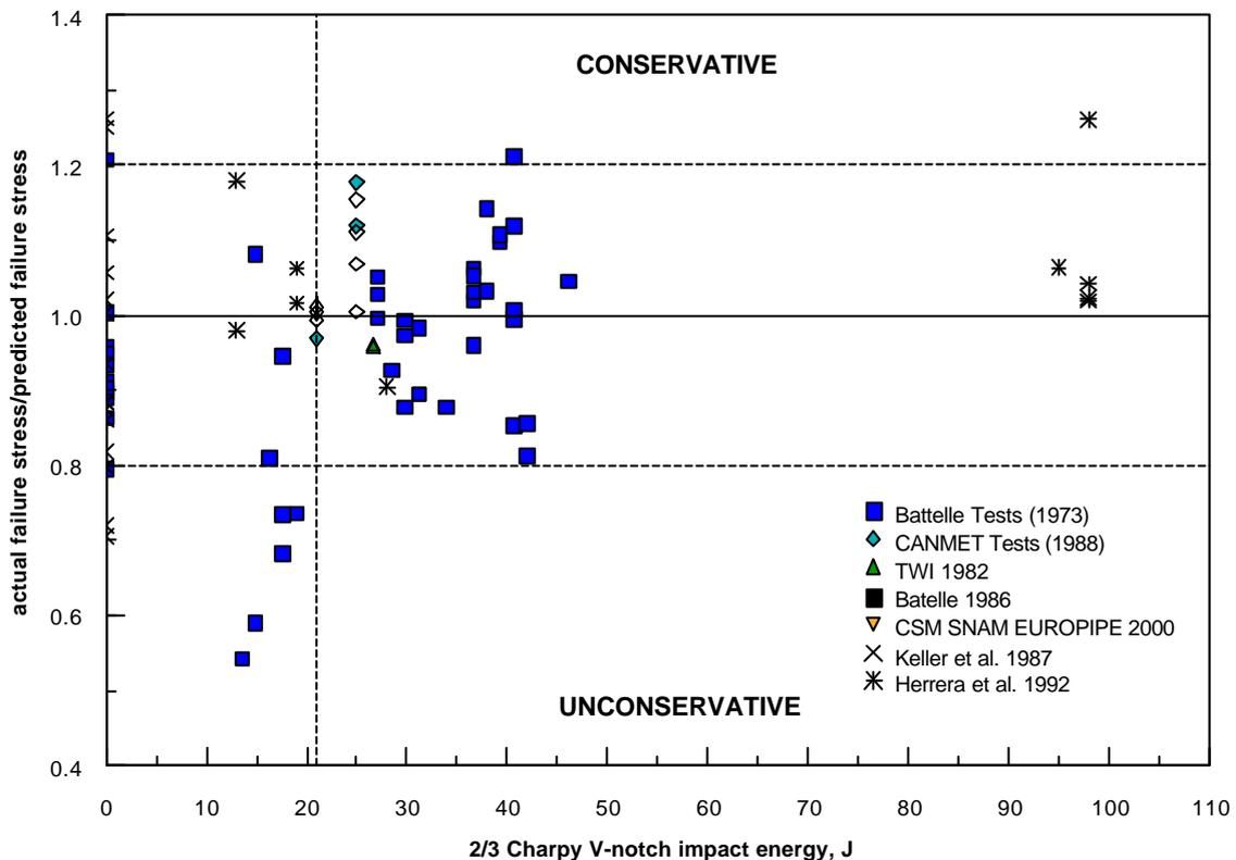
**Figure 5 – The effect of toughness on predictions of part-wall burst tests made using the flow stress dependent part-wall NG-18 equations**
