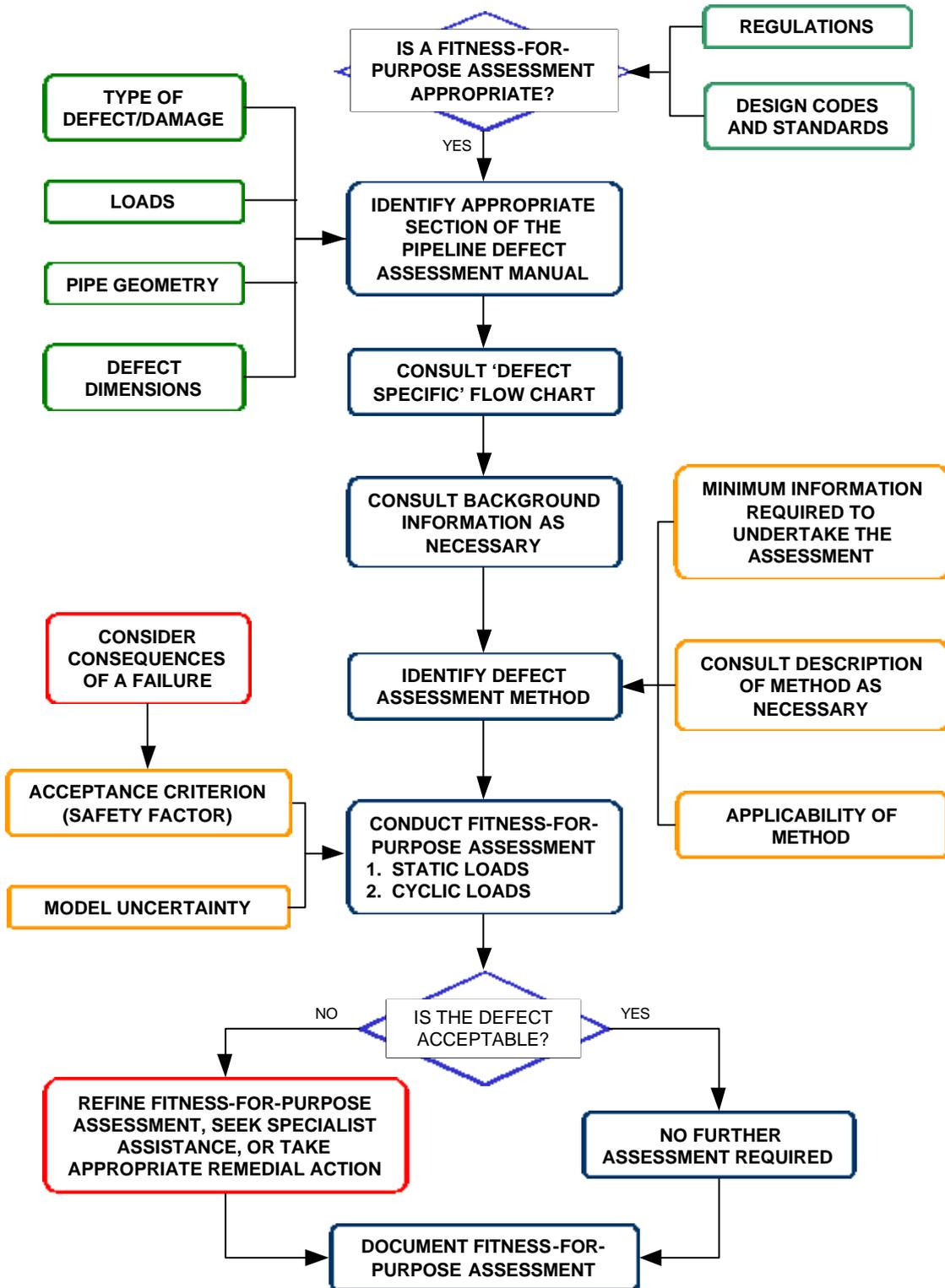
Figure 2 – The fitness-for-purpose assessment of a pipeline defect
