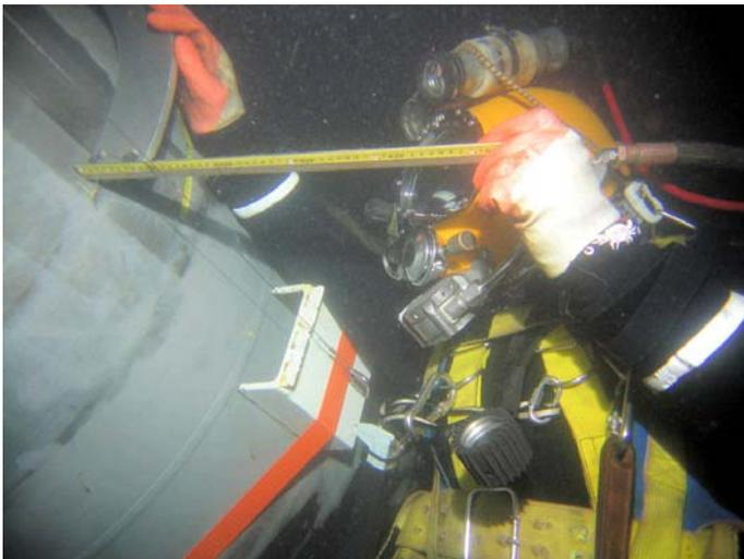
**Figure 6 - Diver Inspection (Taut-Wire)**
