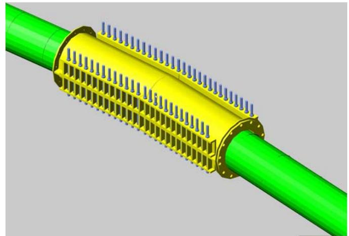
**Figure 10 - Repair Sleeve**
