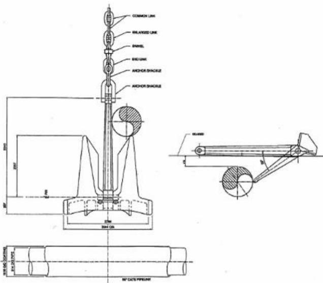
**Figure 9 - Anchor and Pipeline (to scale)**
