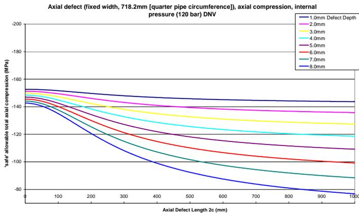
**Figure 4 - Defect Assessment under Axial Compressive Loadings**
