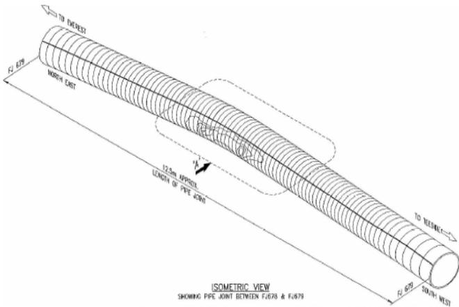
**Figure 8 - Local Deformation**
