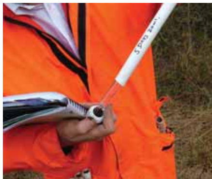
Jet fuel sample in the specially designed 'leak-tube'.
