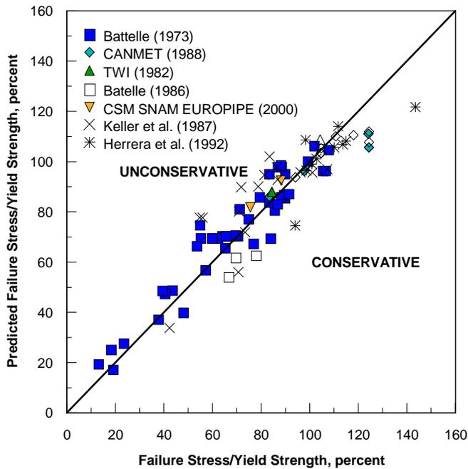
Fig. 4 Failure stress of axially orientated part-wall defects predicted using the part-wall NG-18 equation
