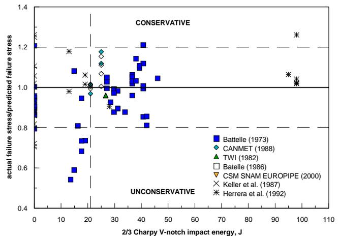
**Fig. 3 The effect of toughness on predictions of part-wall burst tests made using the flow stress dependent part-wall NG-18 equation<sup>6</sup>**
