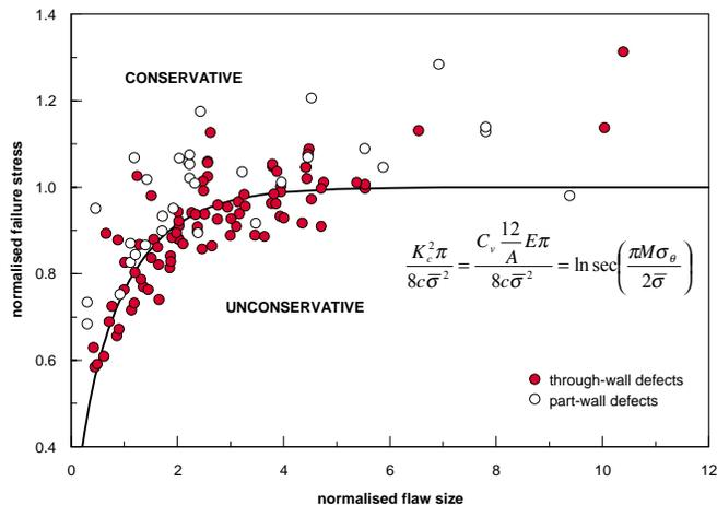
Fig. 1 The NG-18 equations and test data, illustrating flow stress and toughness dependent behaviour<sup>2</sup>
