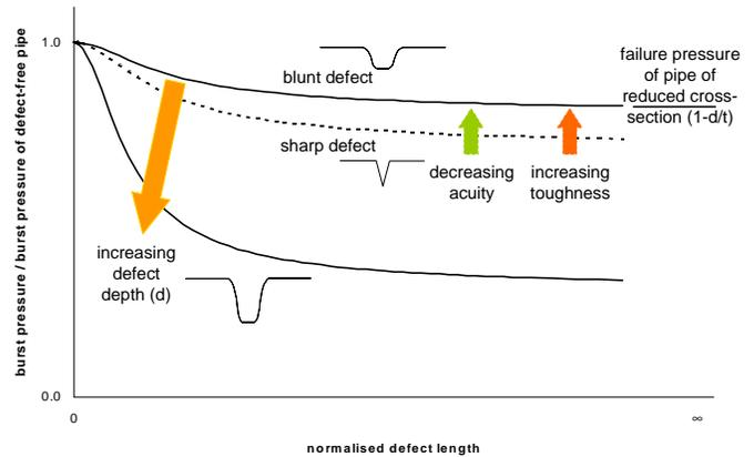
**Fig. 2 The effect of material toughness, defect depth, length and acuity on burst strength**
