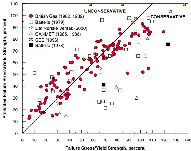
Fig. 7 Failure stress of dent and gouge defects predicted using the semi-empirical dent-gouge fracture model
