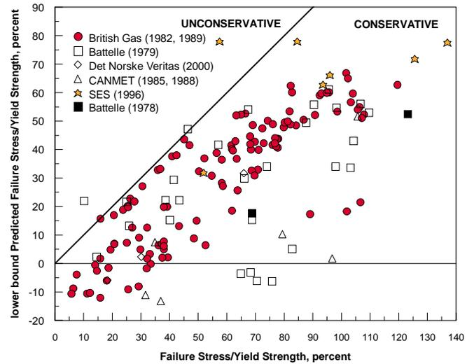
Fig. 8 Failure stress of dent and gouge defects predicted using a lower bound to the semi-empirical dent-gouge fracture model
