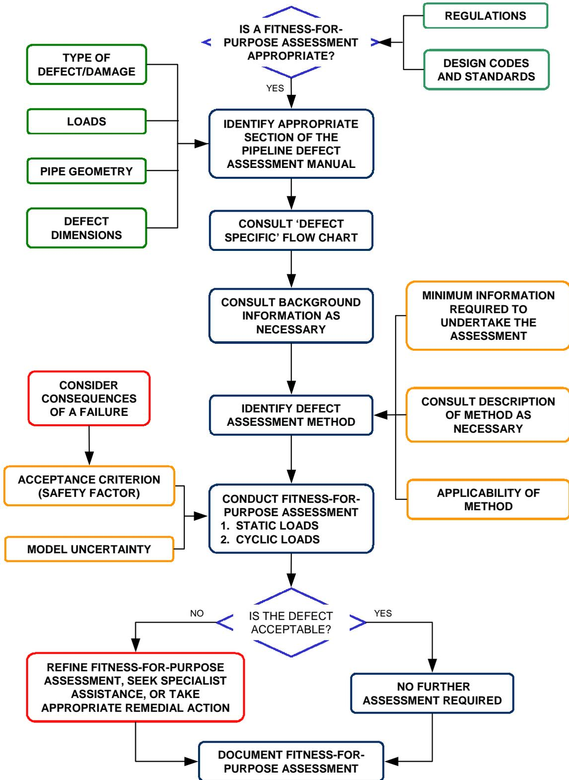
Fig. 9 The role of the Pipeline Defect Assessment Manual in the fitness-for-purpose assessment of a pipeline defect
