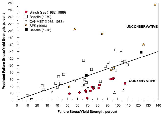
Fig. 6 Failure stress of dent and gouge defects predicted using the empirical Q factor model
