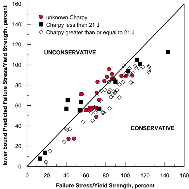
**Fig. 5 Failure stress of axially orientated part-wall defects predicted using a lower bound to the part-wall NG-18 equation**
